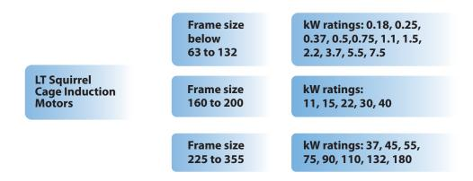
Figure 7: Classification of Sq. cage motors
